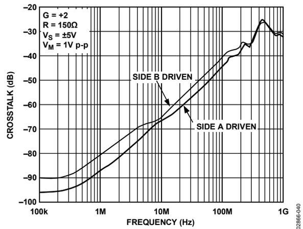
Figure 40. AD8008 Crosstalk vs. Frequency (Output to Output)
