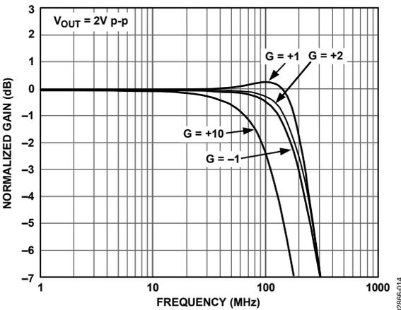
Figure 14. Large Signal Frequency Response for Various Gains
