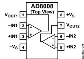
Figure 3. 8-Lead SOIC (R) and 8-Lead MSOP (RM)
