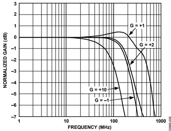
Figure 6. Small Signal Frequency Response for Various Gains
