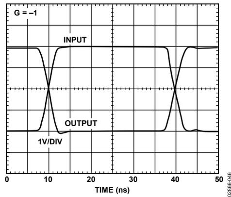
Figure 46. Large Signal Transient Response,  $G = -1$ ,  $R_L = 150\Omega$
